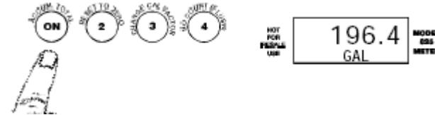
3. Hold buttons ON and 4 for 5 seconds to reset the Accumulated total to '0'
